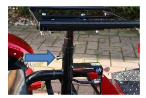
The seat can be assembled from the front by locating the sliders onto the end of the guide rails. It will slide on and stop. By operating the seat adjuster, the final position can be chosen.
